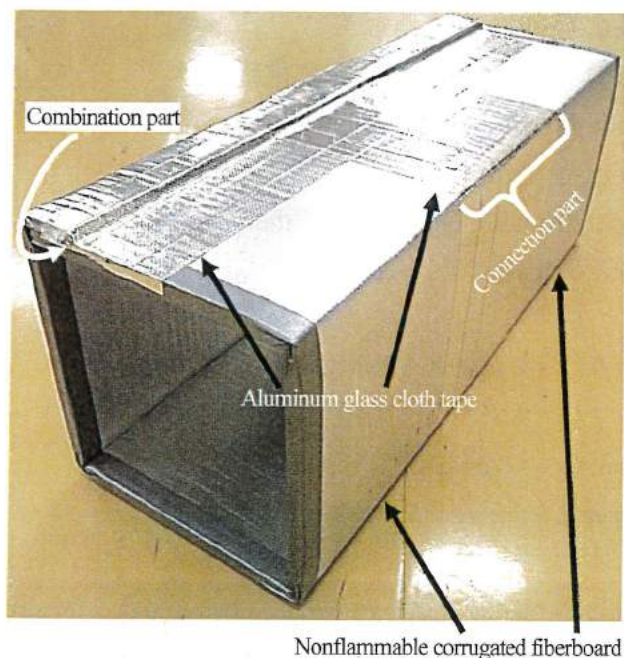
Figure 1 Photo of nonflammable corrugated fiberboard duct
